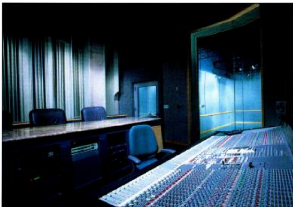
Here a sound-rated door is required to maintain balance with the rest of the facility's sound-isolation performance.
